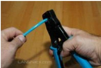
**11.** For Crimping push the connector all of the way in and then squeeze down all the way on the crimper.
